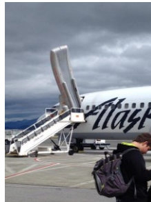
Figure 1. Emergency slide deploys on the ground in an Alaska Airlines Boeing 737-400 (N778AS). Source: Aviation Safety Net (2014)
