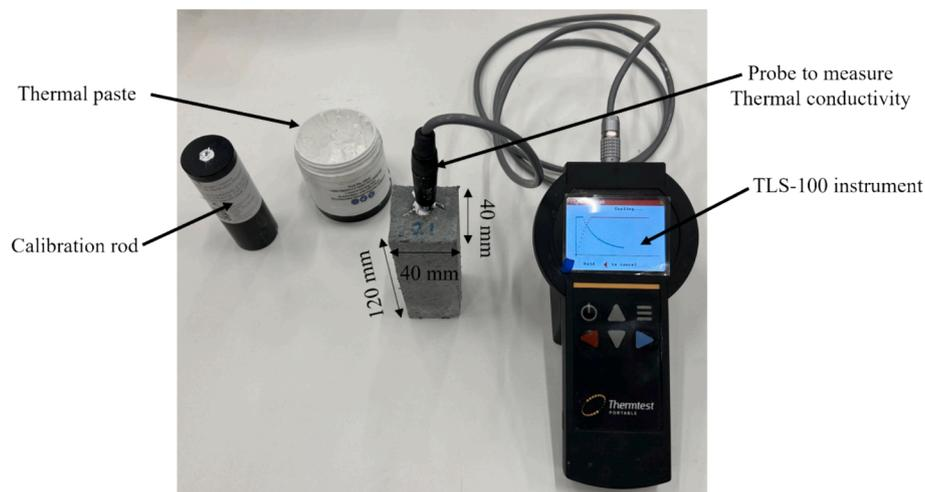
Fig. 2. Thermal conductivity test setup and specimen details.
