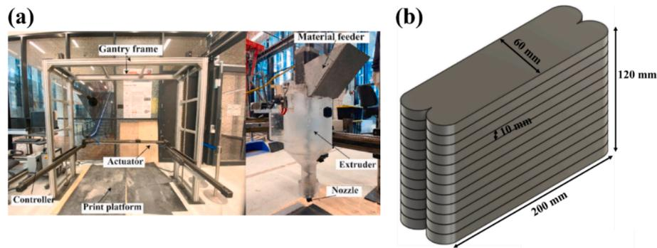
Fig. 1. (a) Gantry type 3D printer (b) Schematic of a printed specimen.
