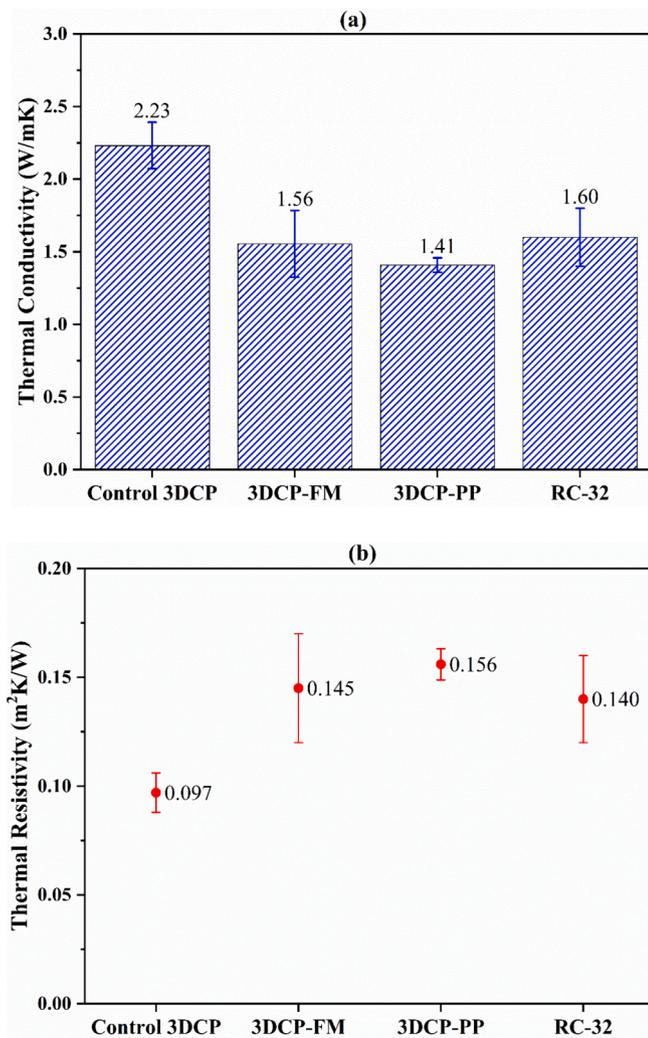
Fig. 4. (a) Thermal conductivity of different wall materials (b) Thermal resistance of the different walls.
