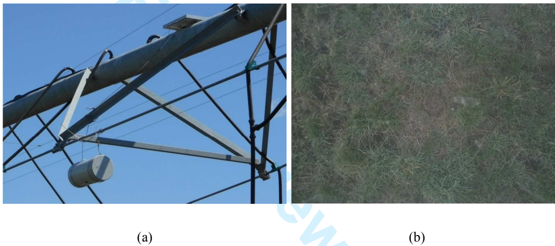
Figure 1. (a) Smartphone units installed on an irrigation machine at the centre of three spans at TIA Dairy Research Farm; and (b) sample image from machine
