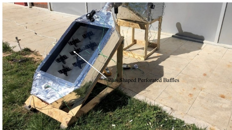
Figure 22. Solar air collector with plus-shaped baffles.
