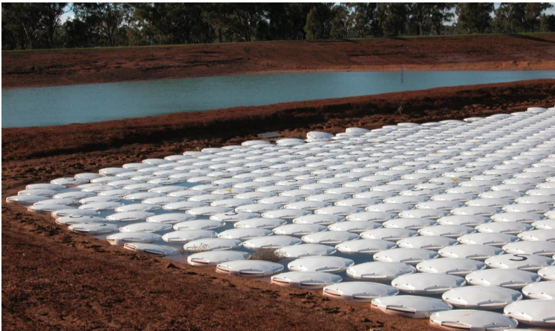
Figure 6: Trial storages at Northparkes Mine, showing one storage covered and the other uncovered.
