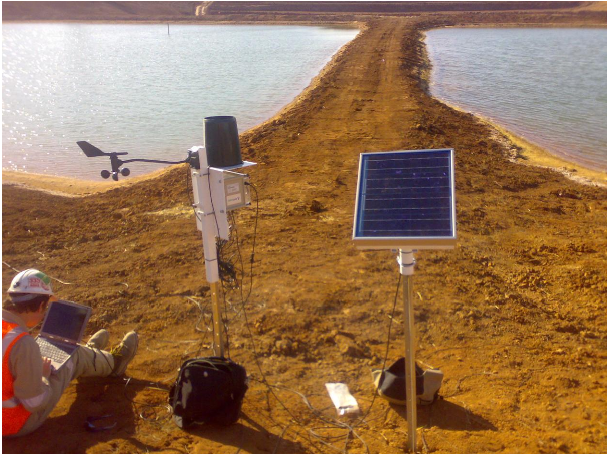
Figure 4: Logger mounted on a pole collecting data from the PST deployed in the water storage.
