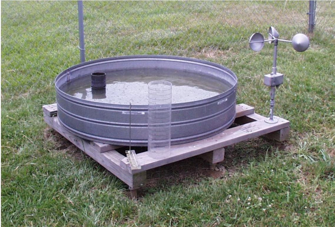
Figure 2: Typical US Class A evaporimeter installation.
