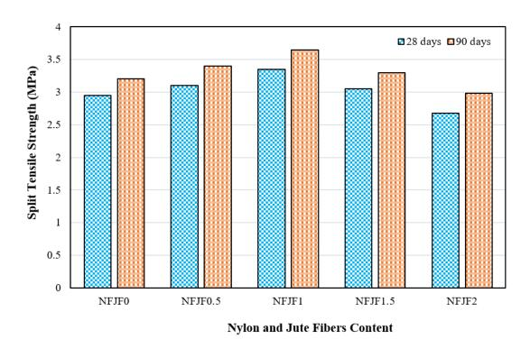
Figure 8. Splitting tensile strength of concrete.
