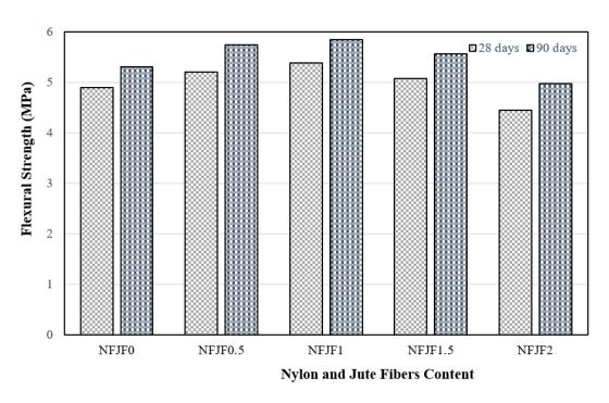
Figure 9. Flexural strength of concrete.
