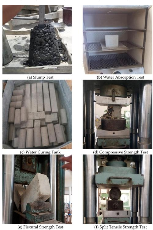
Figure 3. Experimental details of concrete testing.
