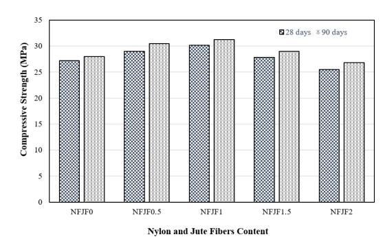
Figure 7. Compressive strength of concrete.
