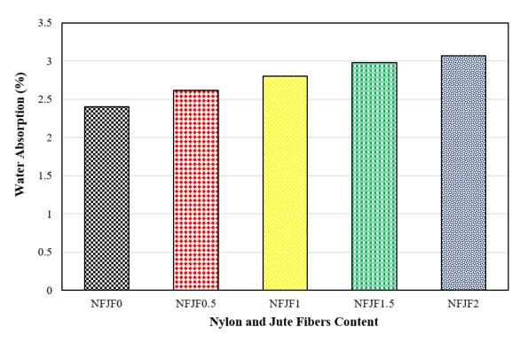
Figure 6. Water absorption of concrete.
