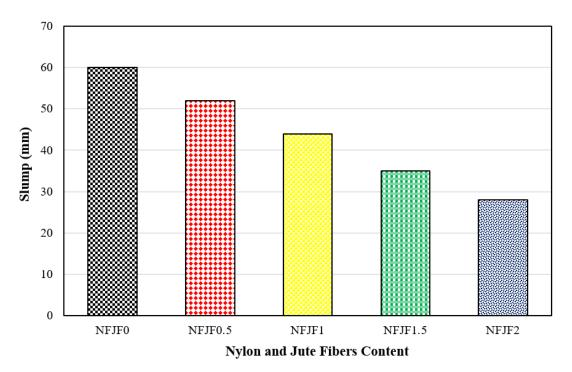
Figure 4. Slump test.
