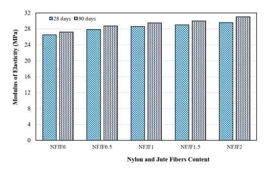
Figure 10. Modulus of elasticity of concrete.
