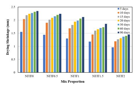
Figure 11. Drying shrinkage of concrete.
