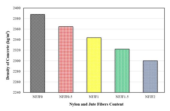
Figure 5. Density of concrete.
