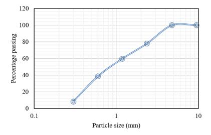
Figure 2. Grading curve of fine aggregate (FA).
