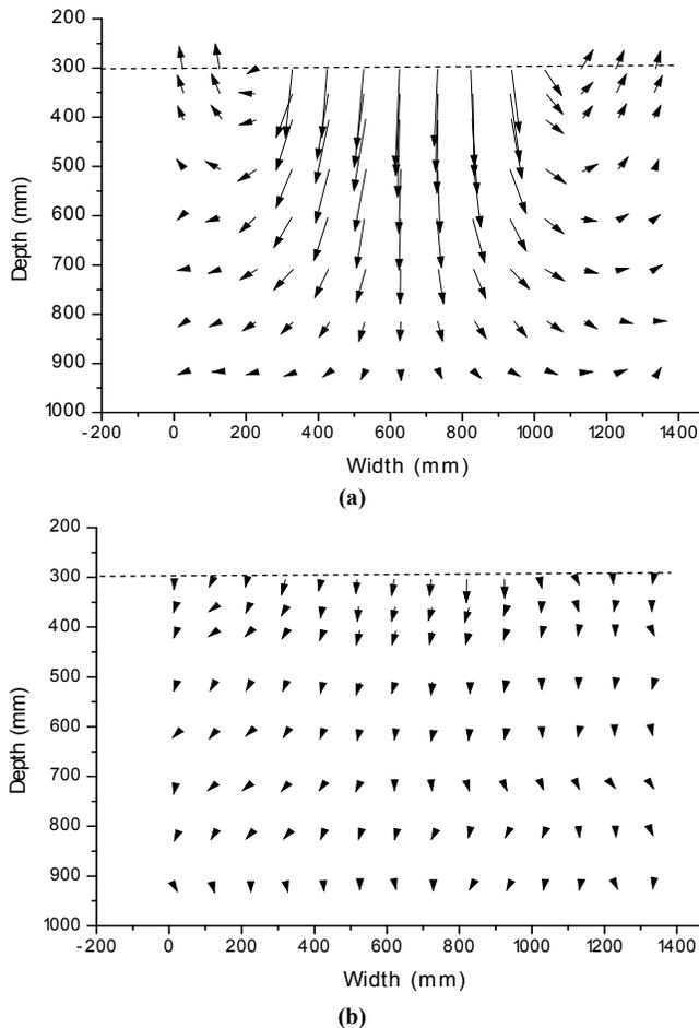
**Figure 3.** Vector diagrams showing the displacement of soil observed beneath the 900/10.5/0.19 tire for (a) low ( $\gamma = 1.20 \text{ g cm}^{-3}$ ) and (b) high ( $\gamma = 1.60 \text{ g cm}^{-3}$ ) initial bulk density soils. The  $x$ -axes indicate the width across the soil bin with the centerline of the tire at approximately 700 mm. The  $y$ -axes indicate the depth in the soil bin. The dotted lines show the soil surface level prior to the tests.
