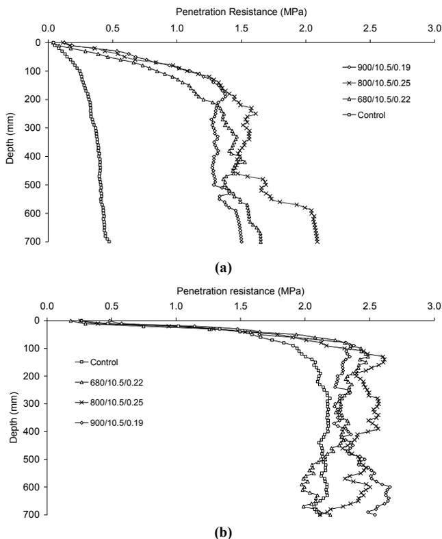
**Figure 6.** Soil penetration resistance with respect to depth corresponding to wheeled and non-wheeled soils for the four central measurements on (a) low ( $\gamma = 1.20 \text{ g cm}^{-3}$ ) and (b) high ( $\gamma = 1.60 \text{ g cm}^{-3}$ ) initial bulk density soils. LSD (5% level) = 0.17 MPa,  $n = 30$ , and  $p = 0.1$ .
