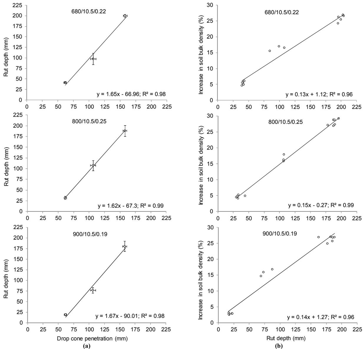
Figure 5. (a) Relationships between drop cone penetration before the pass of the tires over the soil and rut depth at the centerline of wheeling (error bars indicate standard deviations) and (b) relationships between rut depth at the centerline of wheeling and increase in soil bulk density. Sandy loam soil, 10% ( $w w^{-1}$ ) moisture content, uniform soil conditions, and 1.20 to 1.60  $g cm^{-3}$  initial soil bulk densities.
