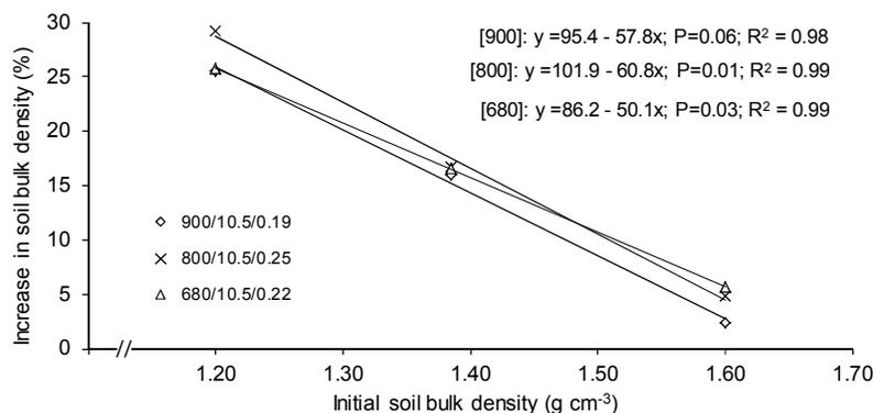
**Figure 4.** Percentage increase in soil bulk density as a function of initial soil bulk density for the range tire configurations used in the soil bin studies using a sandy loam soil, 10% ( $w w^{-1}$ ) moisture content, and uniform soil conditions (corresponding increase in soil bulk density for  $\gamma = 1.40 \text{ g cm}^{-3}$  from Ansorge and Godwin, 2007).
