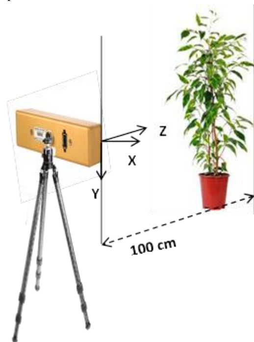
Figure 1. Images are taken from side view of plant with distance of 100 cm between the camera and the end depth of the plant. XYZ represent the camera Cartesian coordinates.
