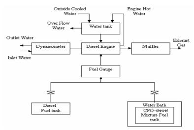
Fig. 1 Schematic layout of the test facilities
