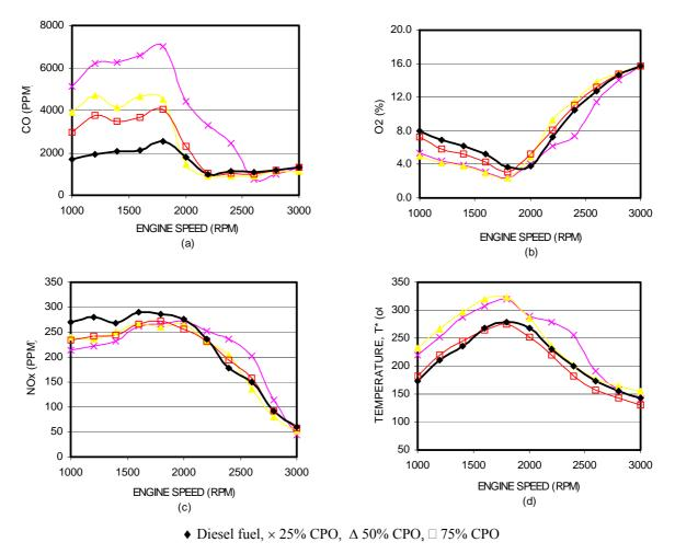
Fig. 3 Exhaust gas analysis
