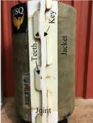
Fig. 1. Novel GFRP jacket with novel joining system.
