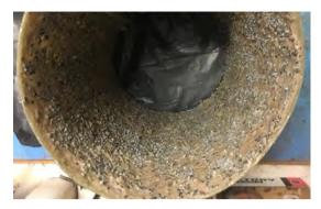
Fig. 4. Roughened GFRP tube.
