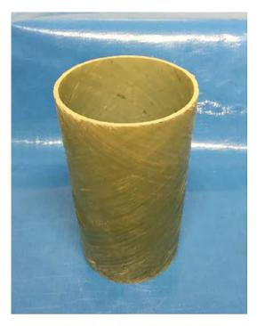
Fig. 1. The pre-fabricated GFRP tube.
