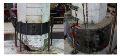
a) Steel collar and anchored steel
