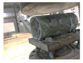
Fig. 2. Splitting tensile test set-up.
