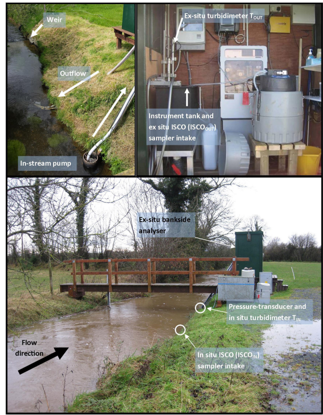
Figure 2. Picture of in situ and ex situ suspended sediment and discharge instrumentation at Grassland B.
