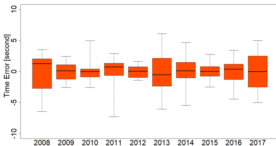
Figure 7. Yearly change of the time error for Electric Reliability Council of Texas (ERCOT) system of North America from 2008 to 2017. One typical month is selected to represent every year. The box-plot depicts the maximum and minimum time error (the ends of the whiskers), the first and third quartiles (the bottom and top of the box), and the mean time error (the band inside the box).
