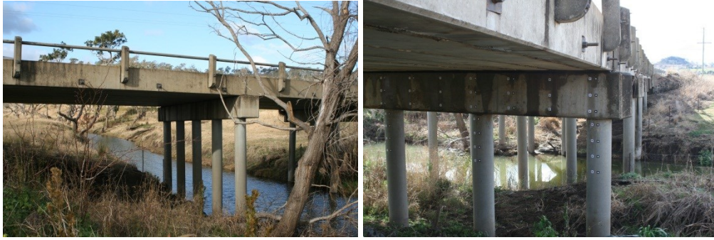
Figure 4. (a). The highway concrete pile bridge vibration testing. (b) The retro-reflective target layout.
