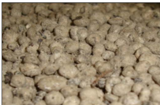
Figure 2: A sample of OMF 15 with particles in the range of 1.18 to 5.60 mm in diameter.
