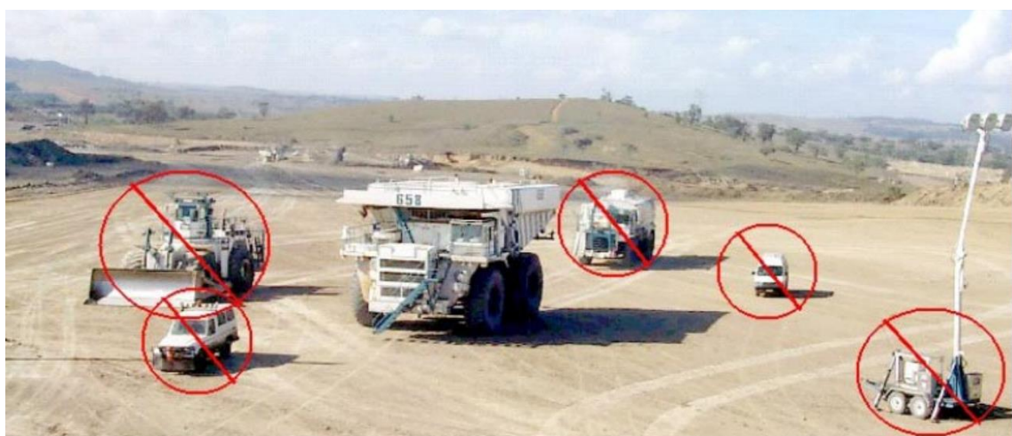
Figure 2-17: Haul vehicle limited visibility from driver’s cab - Source: (Glynn, 2001)
