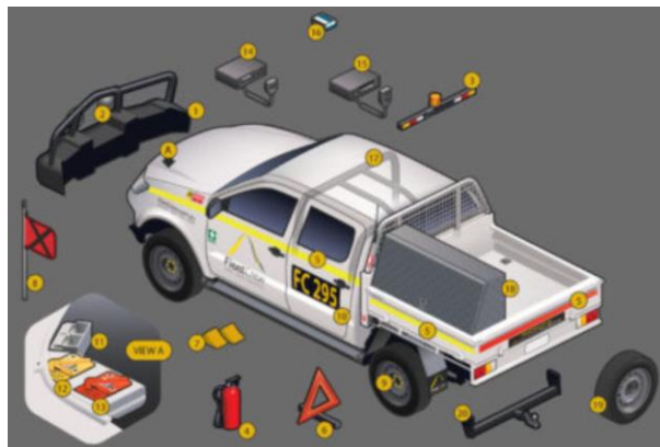
Figure 2-22: Typical mining light vehicle setup – Source: (Fleet Crew, 2021)(Fleet Crew - What Makes a Mine Spec Vehicle Suitable for the Mines? 2021)
