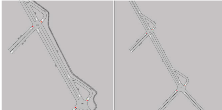
Figure 2-19: Plan view traffic model – separated network (Left) - shared network (Right)
