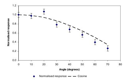
Figure 3 – Comparison of the cosine response of the  $UV_{PGI}$  dosimeter to the cosine curve.
