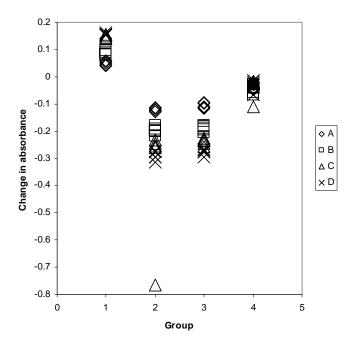
Figure 1 - Side-by-side dot plot of four types of dosimeter, the change in absorbance measured on four sites over four time periods (A, B, C, D) of 30 minutes each, group 1= PS, group 2= NDA, group 3= NDA/PS, group 4= PS/NDA. The change in absorbance was measured at 330 nm.
