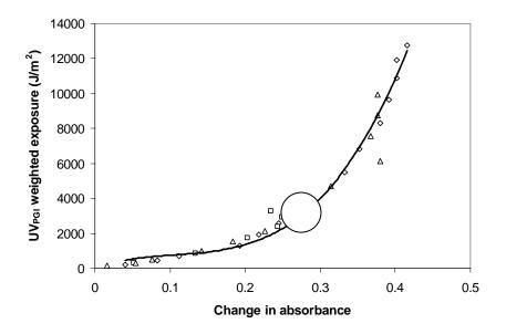
Figure 4 – Calibration of the UV<sub>plant</sub> dosimeter for the measurement of the UV<sub>PGI</sub> exposures. The diamond ( $\blacklozenge$ ) represents the dose response carried out from 10.00am to 3.00pm on 1 February, 2007, the square ( $\blacksquare$ ) represents the dose response carried out from 2.10pm to 5.10pm on 3 March, 2008 and the triangle ( $\blacktriangle$ ) represents the dose response carried out from 9.30am to 1.30pm on 4 March, 2008.
