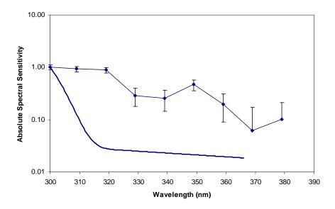
Figure 2 - Spectral response from 300 nm to 380 nm of the  $UV_{PGI}$  dosimeter. The thick line is the PGI action spectrum (Flint and Caldwell, 2003).
