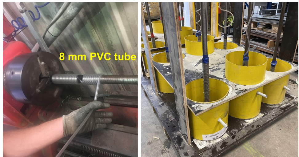
Fig. 4 Preparation of the cylindrical concrete blocks and casting of rifled holes in concrete block using PVC flexible tubes wrapped around the central steel rod
