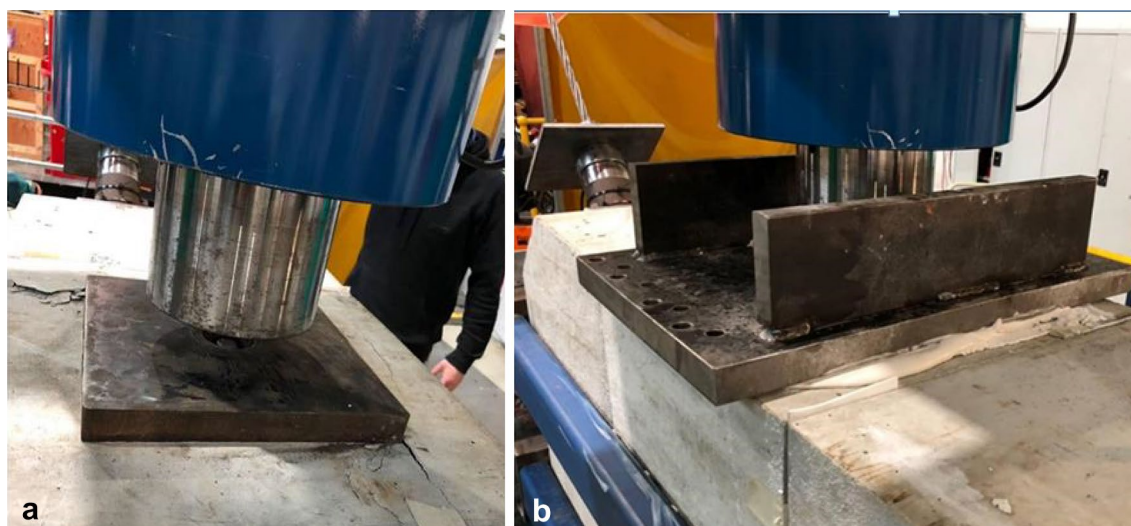
Fig. 10 45 mm diameter cables encapsulated at 45-degree angle being ready for shear testing. a 300 mm 2 loading base plate. b 500 mm × 400 mm loading base plate
