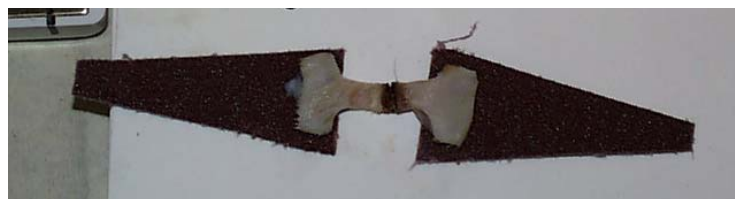
Figure 5-17 Lasered test sample on sand paper prior to mounting in clamps
