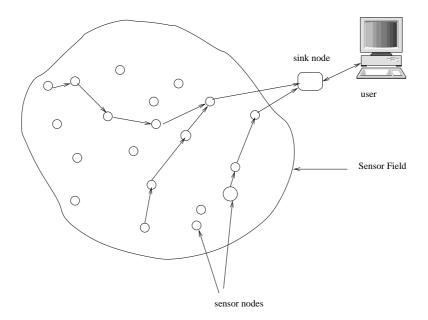
Figure 1: A diagram of a wireless sensor network
