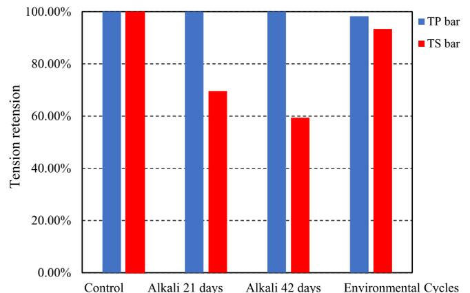
**Fig. 13.** Comparison of durability of thermoplastic bar (TP bar) and thermoset bar (TS bar) [108].
