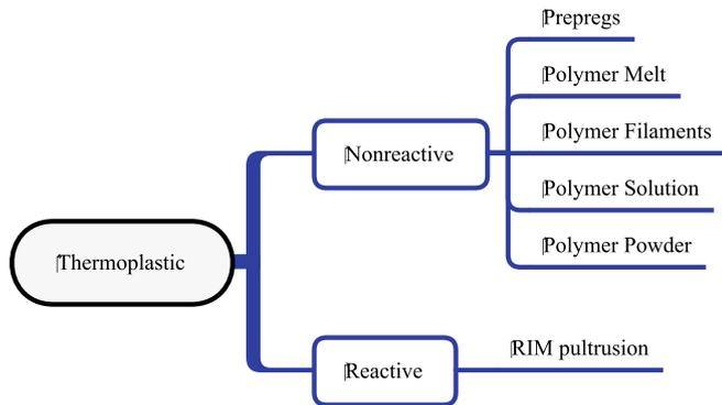
Fig. 4. Thermoplastic pultrusion types.
