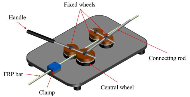
Fig. 8. Bending device for thermoplastic FRP bars [120].
