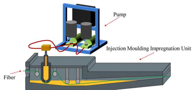
Fig. 6. Reaction Injection Molding (RIM) resin impregnation unit.
