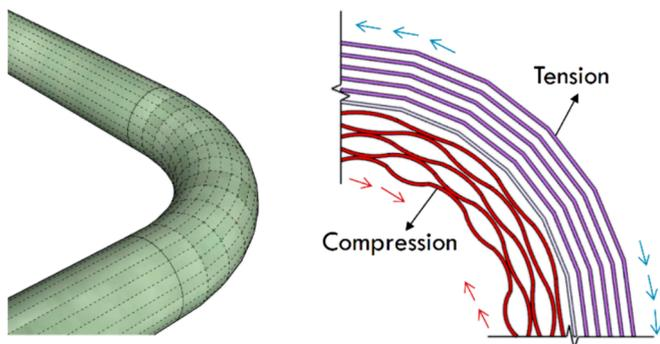
Fig. 1. Fiber squash and stretch in FRP bar reinforcement based on pultrusion.
