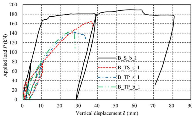
Fig. 19. Applied load versus vertical displacement curves for test beams [145].
