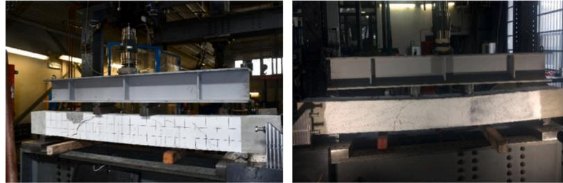
(c) Thermoplastic GFRP straight bars: B-TP-s-1
