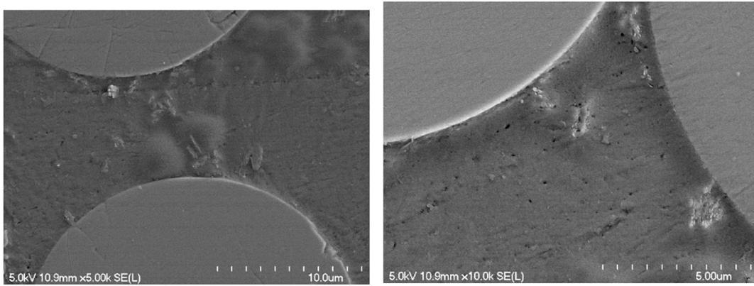
Fig. 15. Micrographs of TP bars at the fiber–matrix interface [51].
