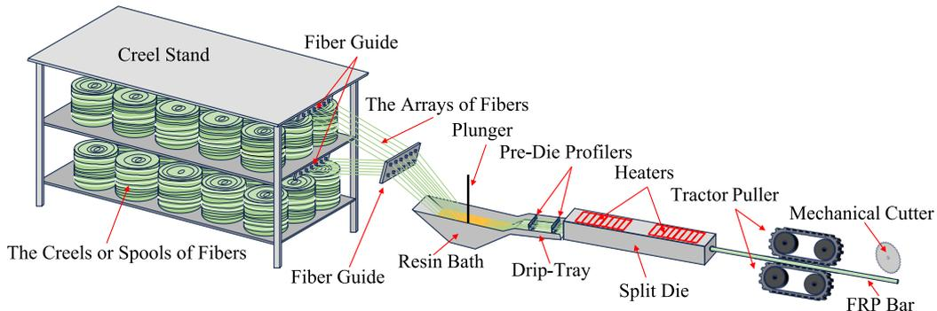
Fig. 5. Non-reactive thermoplastic composite pultrusion process.
