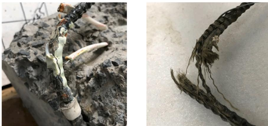
Fig. 9. Typical failure modes in the bending region [120].
