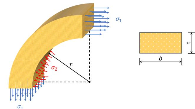
Fig. 10. Stress distribution in the bending part of FRP bending bars in concrete [123].
