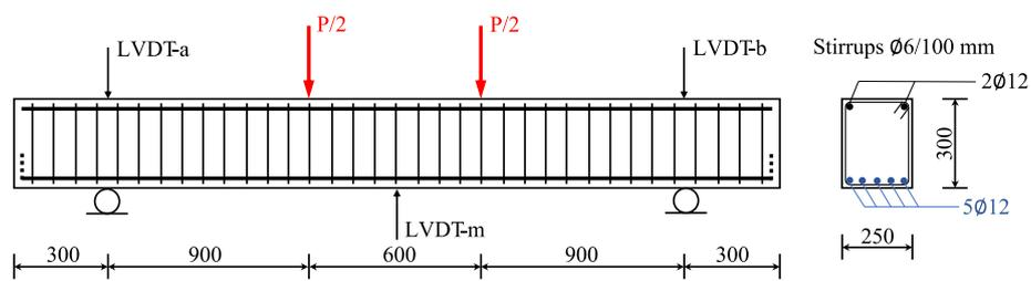
Fig. 17. Geometry of test beam (mm) [145].
