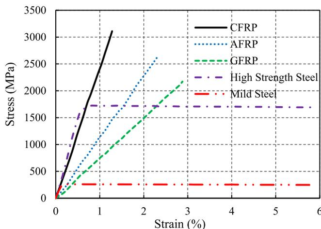
Fig. 3. Comparison of properties between different types of FRP and steel.
