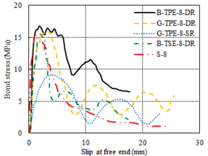
Fig. 12. Parametric comparison of bond stress-slip behavior [120].
