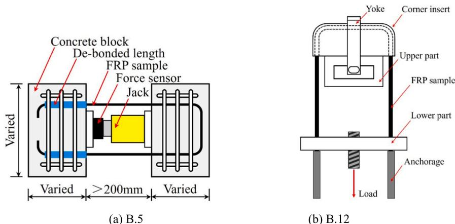
Fig. 7. ACI test methods for bent FRP bars.
