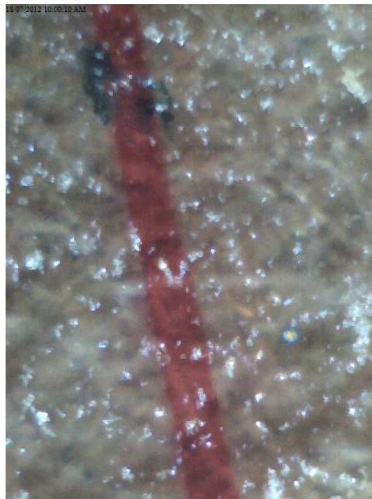
Figure 5.2: Photograph of an ice sampling slide obtained from sampling conditions of 6.5\text{ m/s} flow speed and ultrasonic nozzle water tank pressure of 3.5\text{ bar} .
