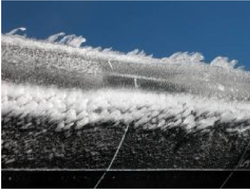
Figure 1.3: Photograph of ice deposits on the wing of the NASA Twin Otter. ( http://www.wearherjackwilliams.com )
