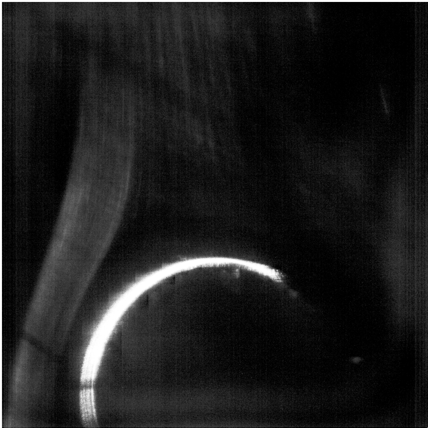
Figure B.1: Air flow streamline at 500 f/s recording rate and flow speed 6.5 m/s.
