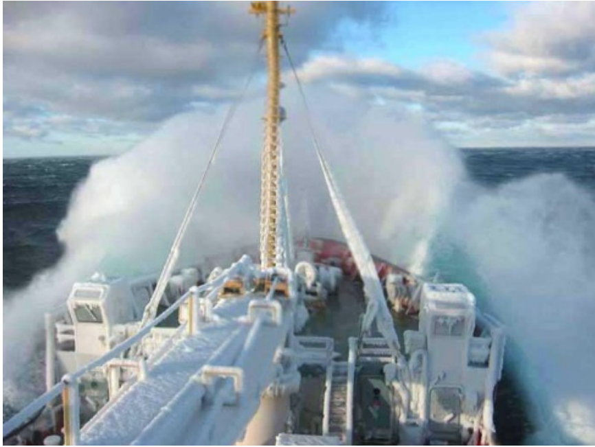
Figure 1.1: Photograph showing ice deposits on surface of a marine vessel and spray which can contribute to ice accretion. (Photo courtesy of the Fishing Vessel Safety Division of the USCG.)
