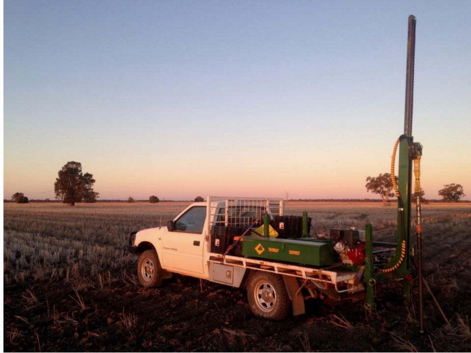
Figure 3.5. Soil coring apparatus
