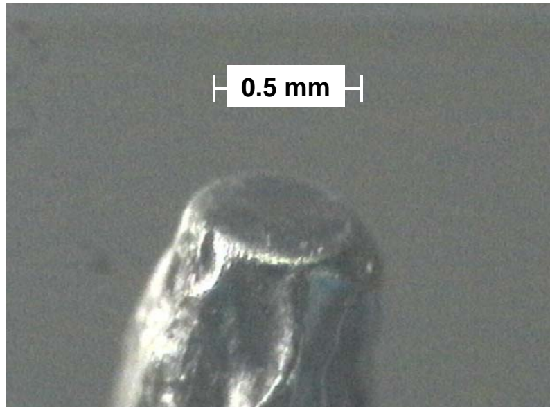
Figure 6.2 Fibre optic pressure sensor made with one hypodermic tube.
