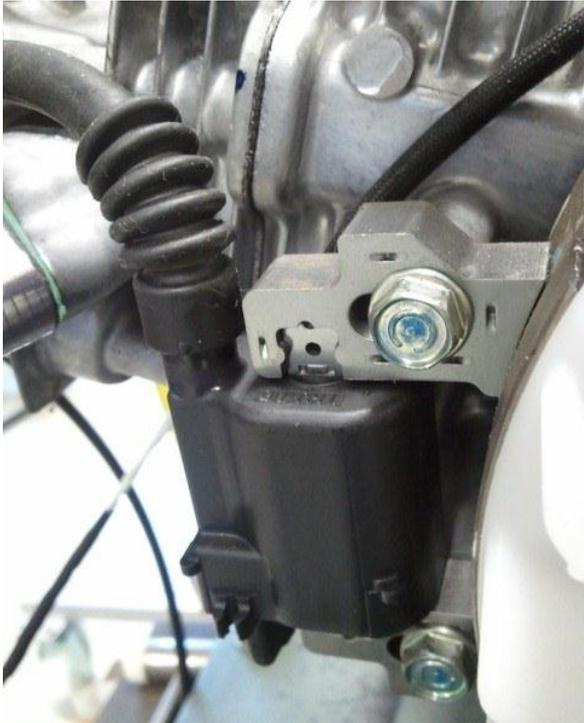
Figure B.7 Old ignition module using TCI system.
