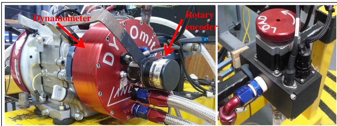
**Figure 6.4** The dynamometer connected to the engine (left) with its controller (right).
