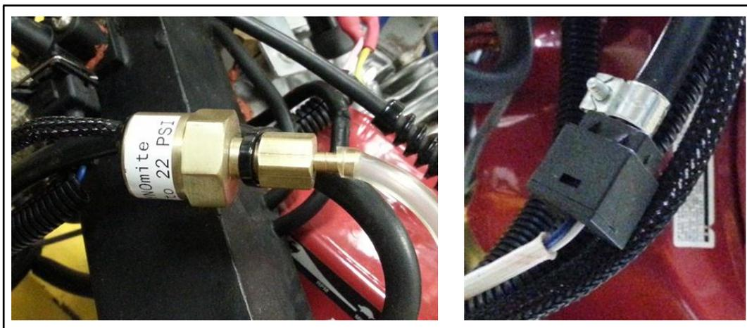
**Figure 6.7** Intake pressure sensors from Land and Sea (left) and for ECU (right)
