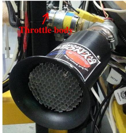
**Figure 6.8** Air flow meter connected to the inlet manifold before the throttle body.
