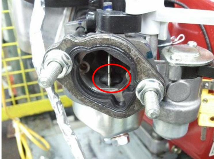
**Figure 6.10** Failure occurred on the plastic part of the fly valve of the carburettor due to the hot air, where the plastic part melted. The carburettor was then removed and replaced with an EFI.
