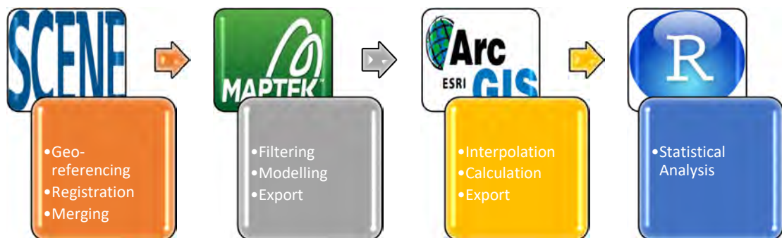
Figure 6-9. Overview of the workflow for the processing and analysis of the terrestrial laser scanning data.
