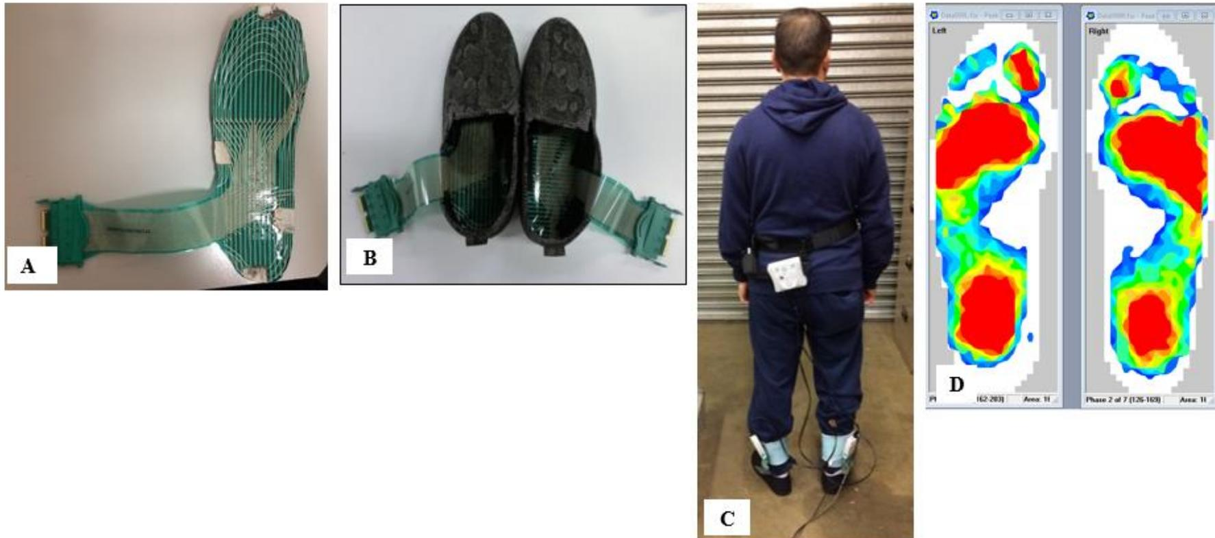
**Figure 3.1.** In-shoe pressure system (pressure sensor). (A) Flexible, thin in-shoe sensors. (B) Inserting the insole system inside the shoe (C) Represents how each participant was set up with the F-Scan system prior to each calibration and recording sensors. (D) Represents a typical plantar pressure recording obtained using the insole system, where high pressure areas can be easily identified.
