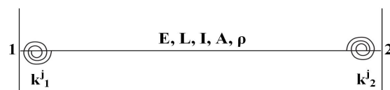
Figure 1. The semi-rigidly connected frame element with rotational stiffness k^j
