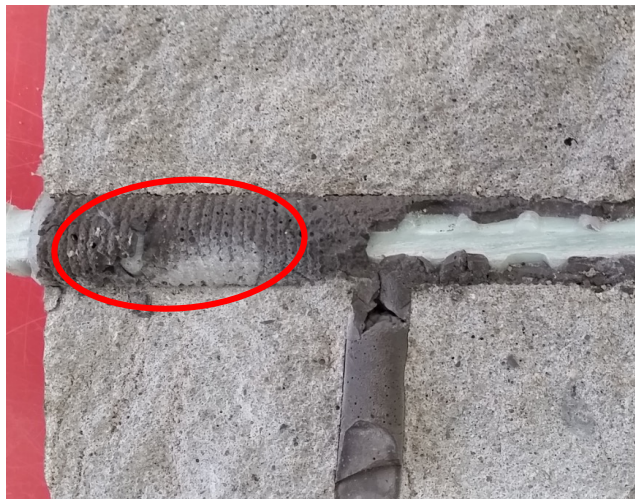
Figure 3.15: Grouting quality examination after testing
