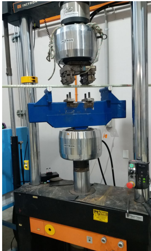
Figure 3.41: Four-point bending test setup of fibreglass rock bolts.
