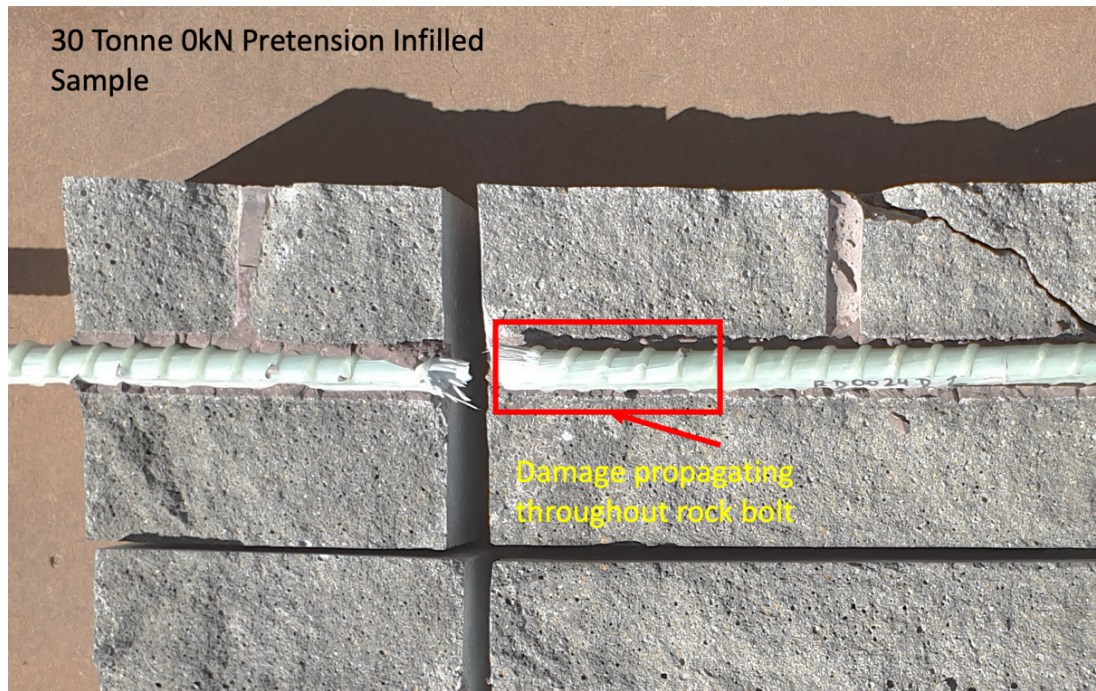
Figure 5.22: Damage propagating through element for 30-tonne rock bolt with 0kN pretension with infilled shear conditions
