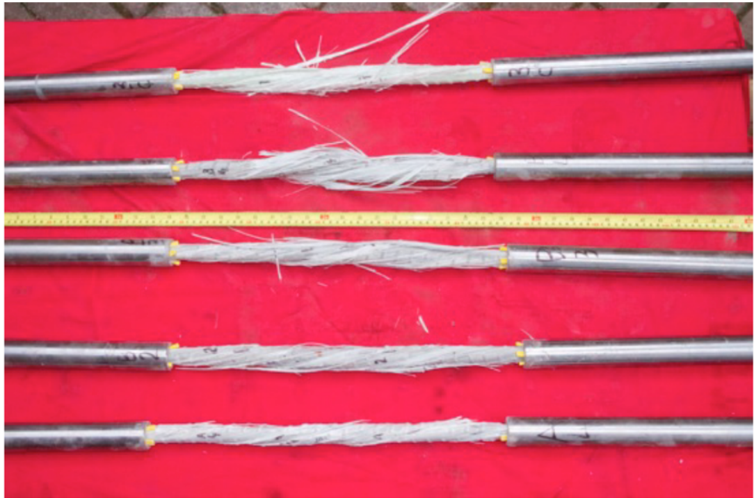
Figure 3.39: Tensile test post failure
