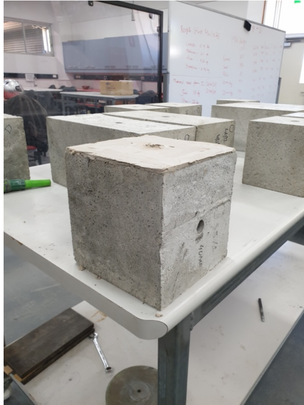
Figure 3.17: Layer of infill material on shearing plane of concrete section.
