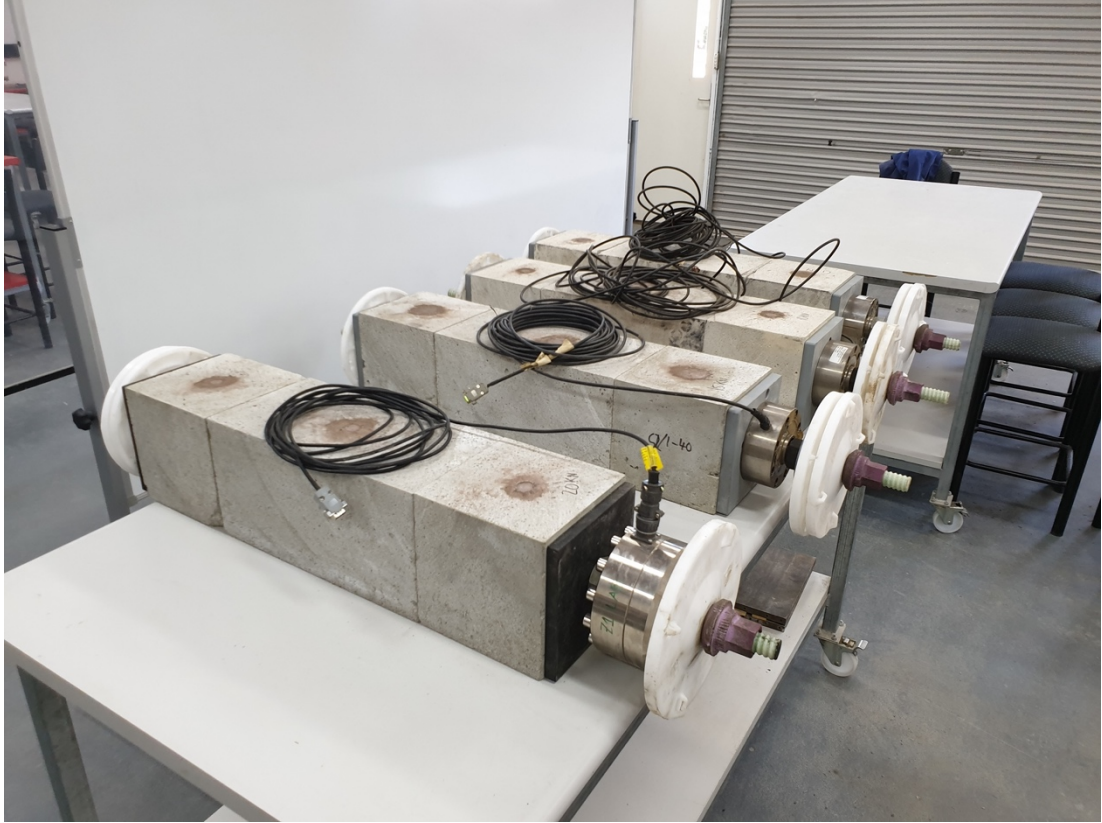
Figure 3.13: Assembled double shear samples.
