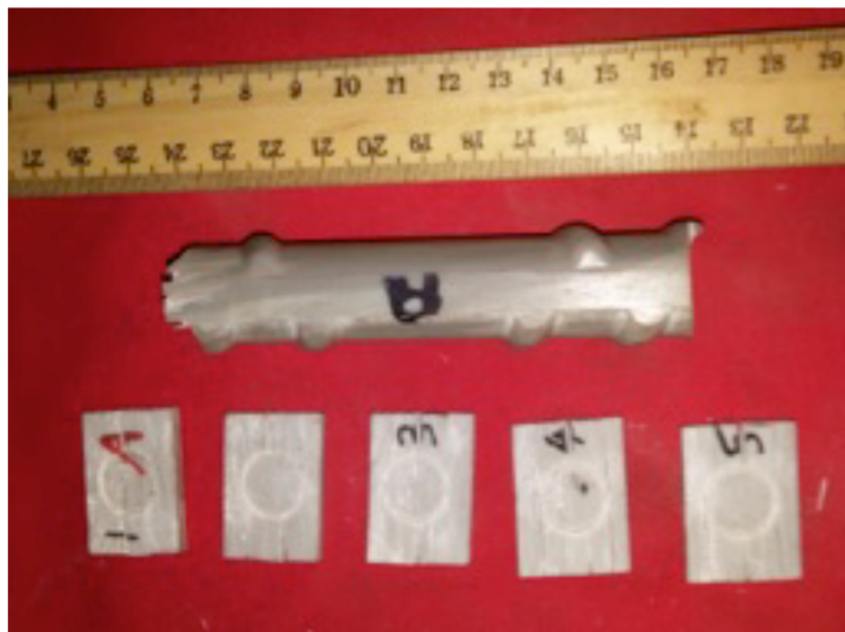
Figure 3.44: Punch test perpendicular fibreglass samples
