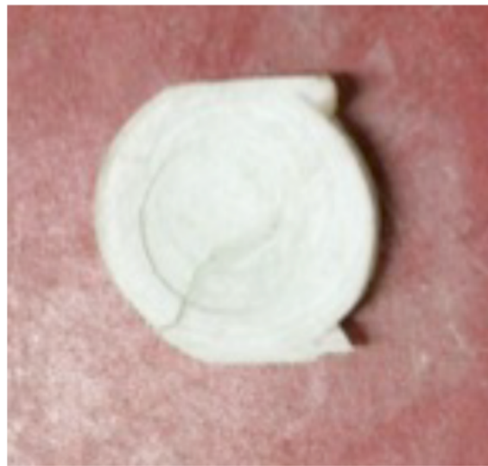
Figure 3.43: Punch test parallel fibreglass sample
