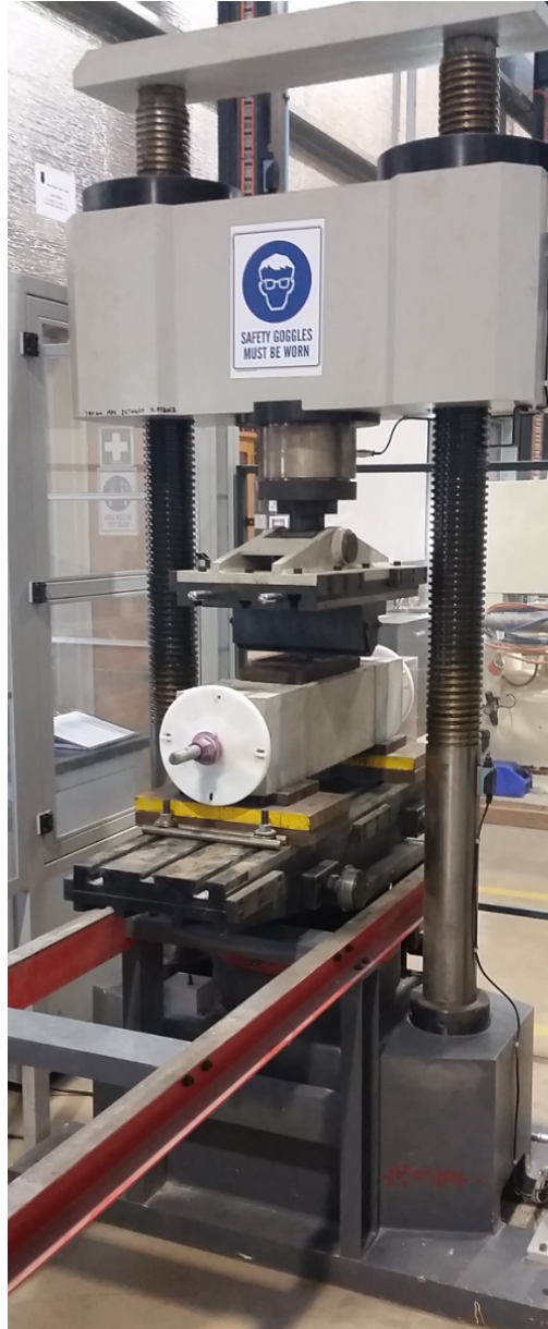
Figure 3.22: Fibre glass bolt double shear testing assembly
