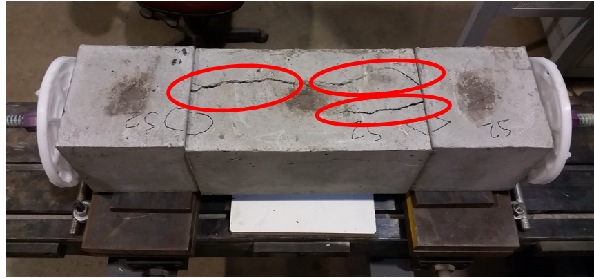
Figure 3.8: Severe damage resulting from a weak concrete matrix.
