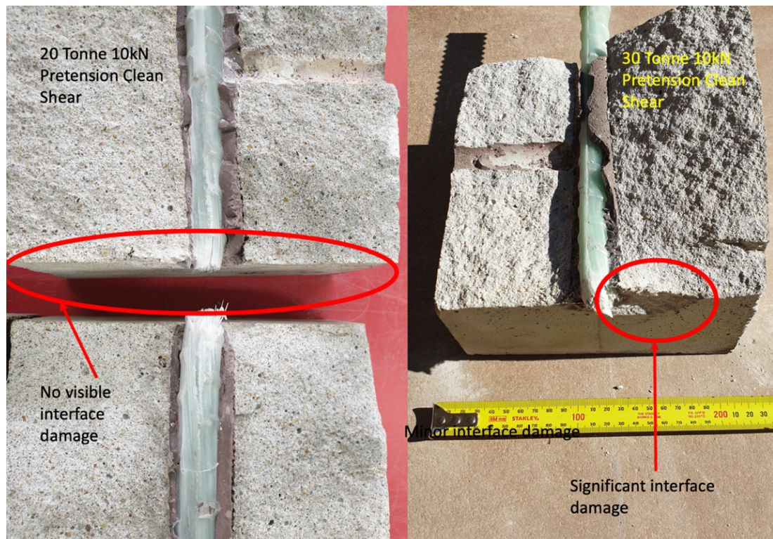
Figure 4.30: Representation of shear plane damage for 20-tonne and 30-tonne rock bolts
