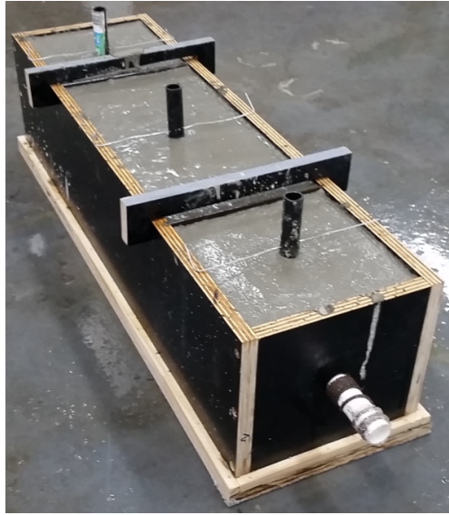
Figure 3.14: Hole positions on top of concrete blocks
