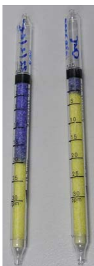
Figure 11. Dräger ® tubes illustrating colour change during measurement (22/2/05)
