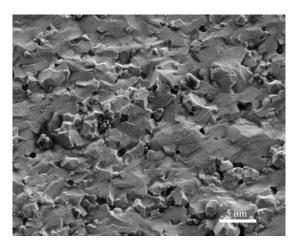
FIG. 2. Microstructure of the fracture of BMT-0.48PT-0.1BZ sintered at
