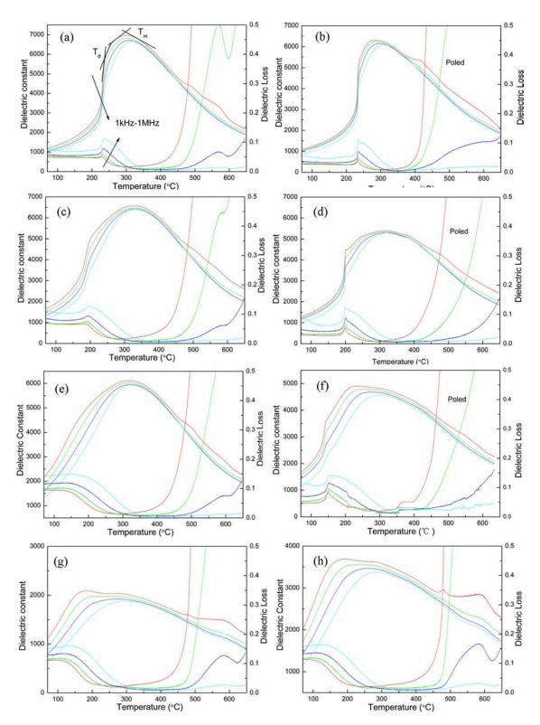
FIG. 6. Dielectric constant and loss as a function of temperature in the frequency range of 1 kHz to 1 MHz for the BMT-xPT-0.1BZ (x = 0.53, 0.5, 0.48, 0.47, and 0.45). (a), (c), (e), (g), and (h) are data for the unpoled ceramics, while (b), (d), and (f) are data for the poled ceramics.
