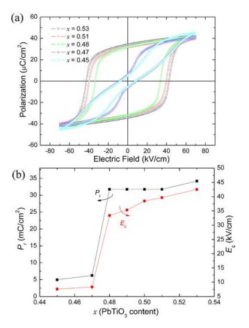
FIG. 3. (a) P(E) loops and (b)  $P_{\rm r}$  and  $E_{\rm C}$  for the BMT-xPT-0.1BZ with  $0.45 \le x \le 0.53$ .
