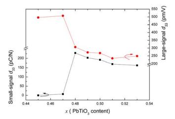
FIG. 5. Small and large-signal  $d_{33}$  for the BMT-xPT-0.1BZ with  $0.45 \le x \le 0.53$ .
