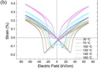
FIG. 7. Temperature dependence of (a) P(E) and (b) S(E) curves for the BMT-0.48PT-0.1BZ.
