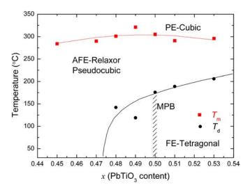
FIG. 8. Phase diagram of BMT-xPT-0.1BZ.
