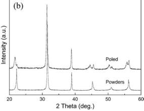
FIG. 1. (a) X-ray diffraction patterns of crushed ceramic powder of BMT-xPT-0.1BZ (0.45  $\leq x \leq$  0.53) at room temperature; (b) x-ray diffraction patterns of crushed ceramic powder and a poled ceramic pellet for the composition of BMT-0.48PT-0.1BZ.
