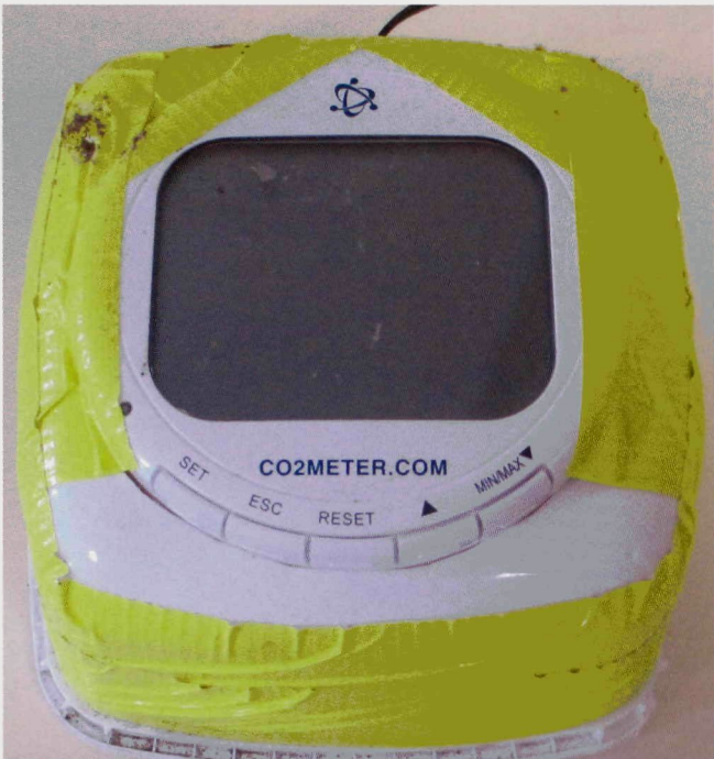
Figure 3: Top view of the gas capture hood with the CO 2 measurement meter fixed into the centre.
