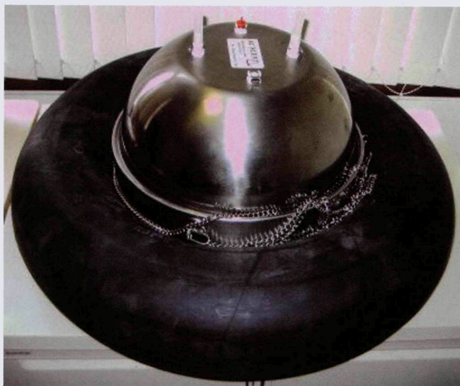
Figure 1: A gas capture hood designed to enclose GHGs from both solid and liquid surfaces.
