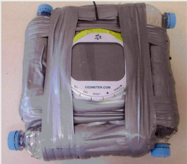
Figure 5: Top view of the gas capture hood with the CO 2 measurement meter fixed into the centre and the empty water bottles attached to the outside.
