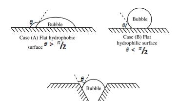
Case (C) conical cavity
