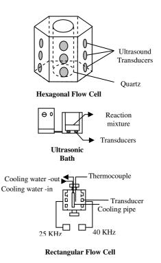
Figure 2. Three designs of cavitation reactors that are broadly used (reproduced from the literature [58])
