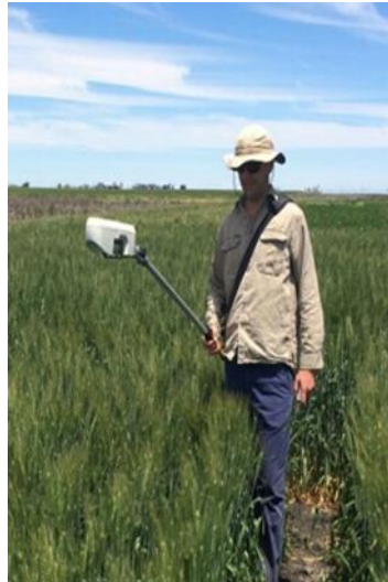
Figure 4.1 The Greenseeker™ positioned above a plot assessing wheat for tolerance to Pratylenchus thornei at a dedicated field research site (Source: Stephen MacDonald, USQ).
