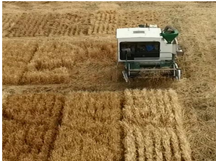
Figure 2.7 An experimental-plot header harvesting grain to determine cultivar tolerance to Pratylenchus thornei by grain yield (Source: Adam Quade, Queensland Department of Agriculture and Fisheries).
