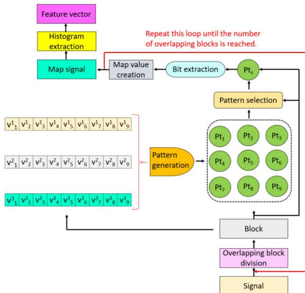
**FIGURE 4.** Block diagram of the 3LBP feature extraction function. **\*\*Pt**, pattern; **Pts**, selected pattern; **v**, value within each signal block.
