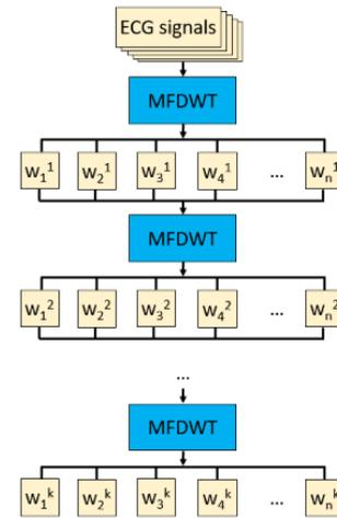
**FIGURE 3.** Block diagram of the MFMDWT.
