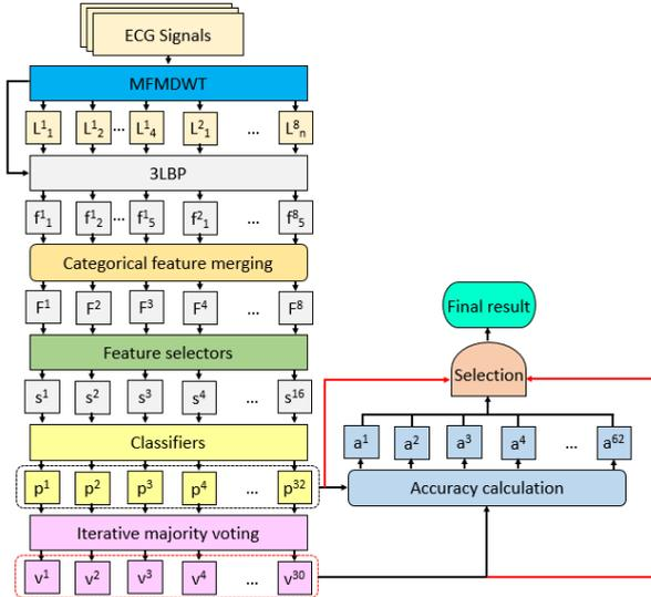
**FIGURE 2.** Block diagram of the proposed feature engineering model. \*\*w, wavelet sub-band; f, feature vector generated by 3LBP function; F, merged feature vector; s, selected feature vector; p, prediction vector; v, voted prediction vector; a, calculated accuracy.
