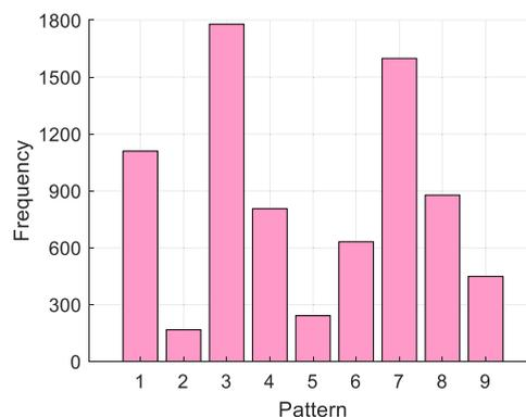
FIGURE 6. Frequency distribution of 3LBP-generated patterns used for an example ECG segment.
