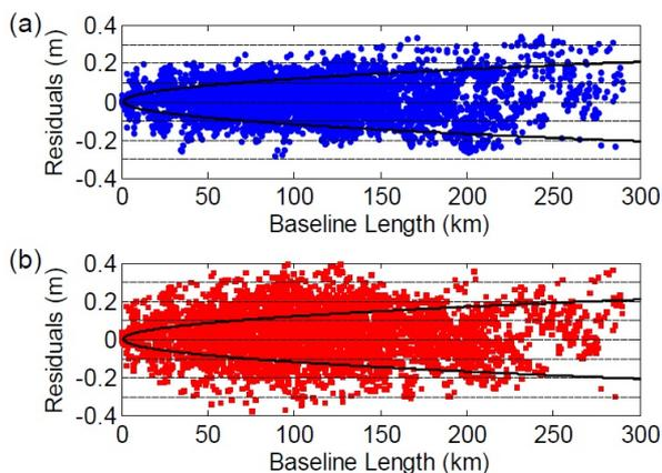
**Figure 4:** Snowy Mountains residuals between (a) AUSGeoid09- and (b) AUSGeoid98-derived and official AHD height differences over 5,356 possible vectors. The unbroken line describes the allowable 3<sup>rd</sup> order differential levelling misclose.
