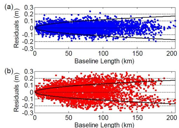
**Figure 3:** Mid Hunter residuals between (a) AUSGeoid09- and (b) AUSGeoid98-derived and official AHD height differences over 3,320 possible vectors. The unbroken line describes the allowable 3<sup>rd</sup> order differential levelling misclose.
