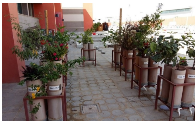
Figure 2 The 36 biofiltration columns.
