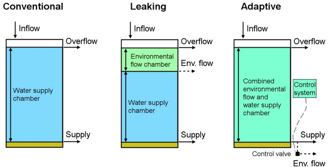
**Fig. 1-1** Rainwater tank storage arrangements with alternatives for environmental flow. Note that with the leaking scenario, a physical partition between chambers is not necessary but this virtual separation is defined by the fixed position of the gravity-draining environmental flow outlet.
