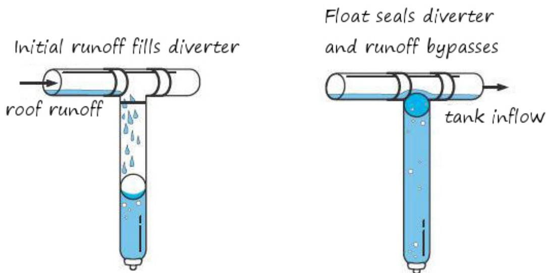
**Fig. 2-5** Rainwater harvesting first flush device. Original source unknown.
