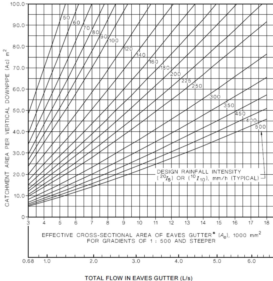
**Fig. 2-3** Required size of eaves gutters for gradients of 1:500 and steeper. Source: (AS 3500.3 2003)
