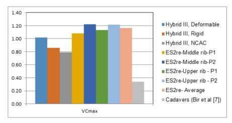
Figure 10: VCmax values for LP\_20 impact condition
