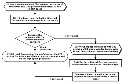
Figure 1: Procedural steps to evaluate the suitability of the ATDs for ballistic impacts
