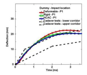
Figure 3: Dynamic chest deflection of the Hybrid III thoraces (LP 20 impact condition)
