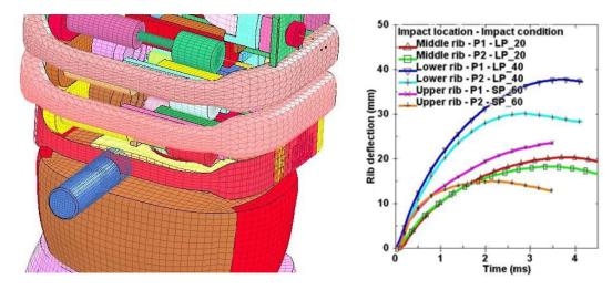
**Figure 13:** ES-2re subjected to LP\_40 impact condition (Lower rib – P1 location)
