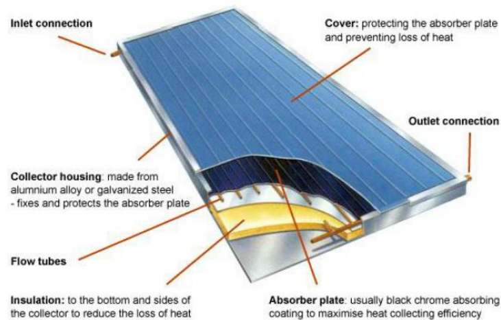
Figure 1: A typical flat plate collector, (Source: GreenSpec, 2010)
