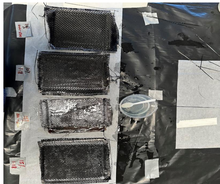
Figure 4. Fabrication of sandwich structure of composite.
