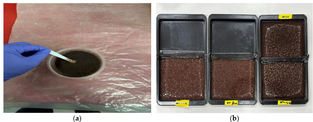
Figure 2. (a) Making of the slurry (mixing: resin, hardener, and nutshell); (b) moulds with slurry (kept at room temperature for curing).
