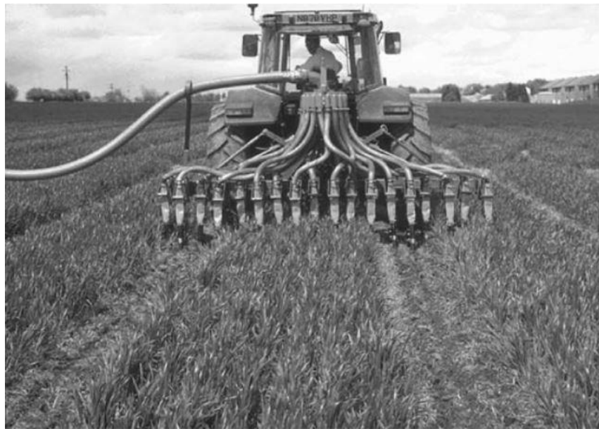
Figure 2-32: Umbilical hose system (Pullen, Godwin, Grundon, & Hann, 2004)
