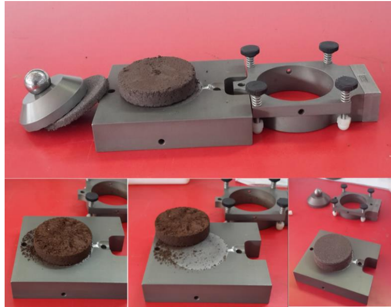
Figure 3-34: Undisturbed soil filling the upper half, while the bottom half was filled with a circular steel block to measure adhesion and soil-metal friction angle
