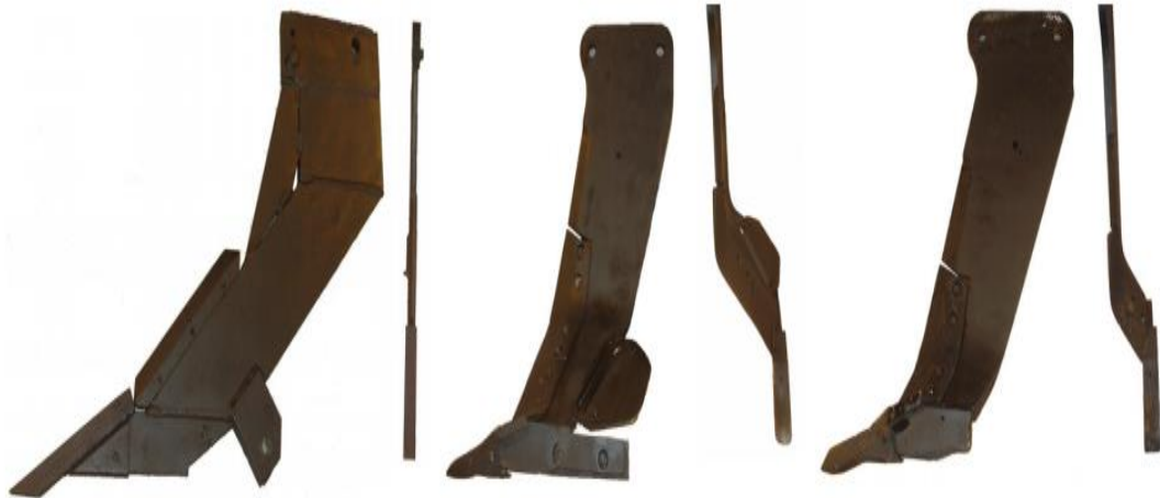
Figure 2-17: Side and front views of KMC subsoiler (left: angled shank (45°) with 2.5 and 4.4 cm of shank and tip width respectively), BBP subsoiler (centre: bentleg shank (45°) with the leading edge rotated forward by 25° with 2.5 and 5.7 cm of shank and tip width respectively and >21.6 cm width contacts with soil as shank travelled forward), and BBT subsoiler (right: bentleg shank (45°) and a slightly narrower version of BBP with 2.5 and 7.5 cm of shank and tip width respectively and >12.7 cm width contacts with soil as shank travelled forward) (Raper et al., 2005)
