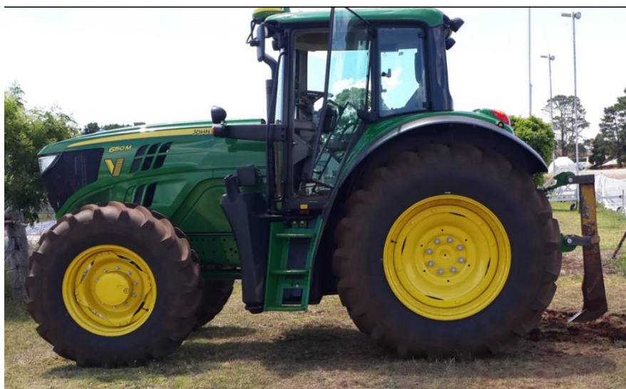
Figure 3-5: Machinery unit (JD 6150 M with Barrow single tine ripper) during ripping operation at Ag plot site, Toowoomba
