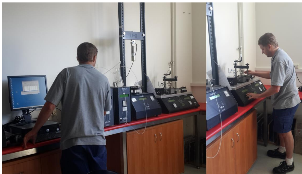
Figure 3-29: Direct shear test (ShearTrac-II), Z1 Lab, USQ
