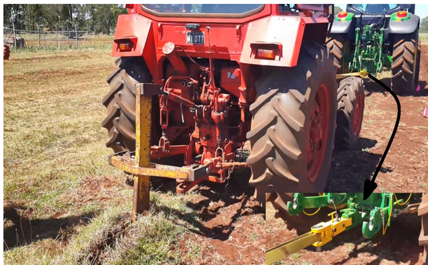
Figure 3-7: JD 6150 M, pull meter, Belarus 920, and Barrow single tine ripper (respectively) during the draft force procedure, Ag plot site
