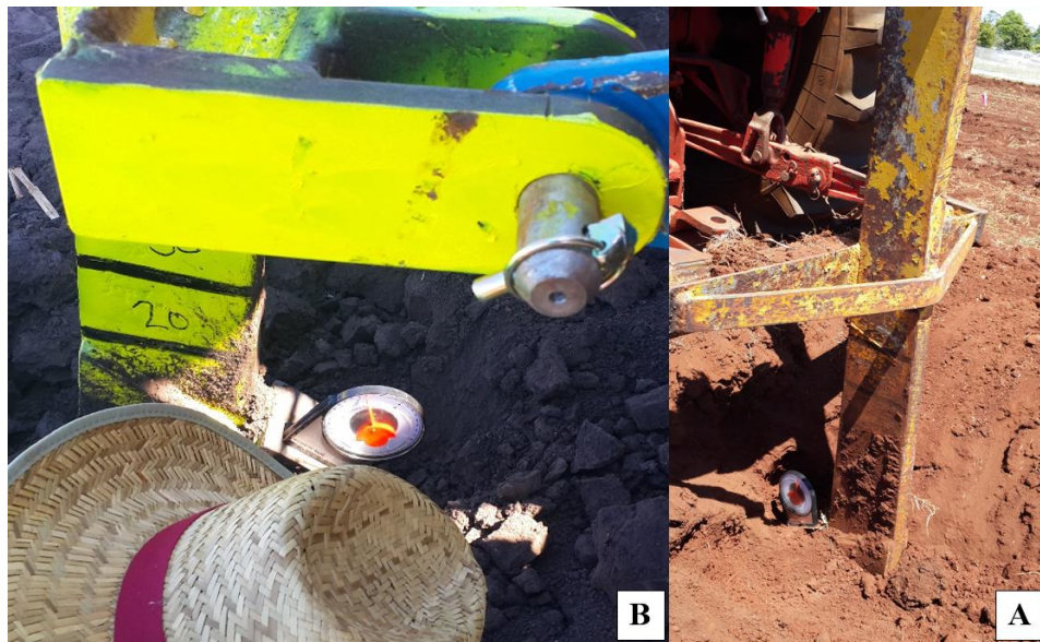
Figure 3-32: Measuring the tip rake angle via dial gauge with magnetic base while the ripper is penetrating the soil at each operation depth at: (A) Ag plot site, (B) Evanslea site
