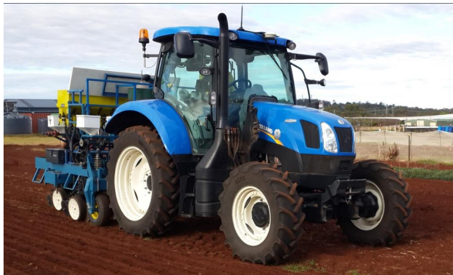
Figure 3-10: Machinery unit (New Holland T6.150 with Big Rig seeder) during wheat sowing operation at Ag plot site
