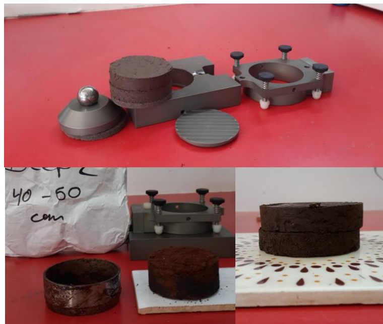
Figure 3-33: The undisturbed soil filling the direct shear box to measure cohesion and internal friction angle
