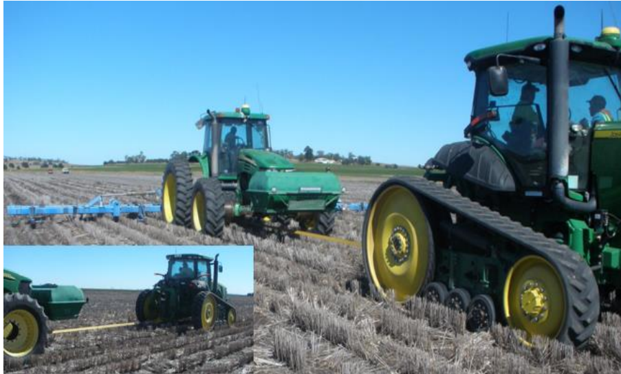
Figure 3-8: JD 8310 RT, pull meter, JD 7920 and Tilco eight tines ripper (respectively) during the draft force procedure, Evanslea
