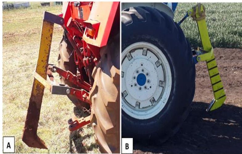
Figure 3-27: Barrow single tine ripper at (A) Ag plot site, (B) Evanslea site
