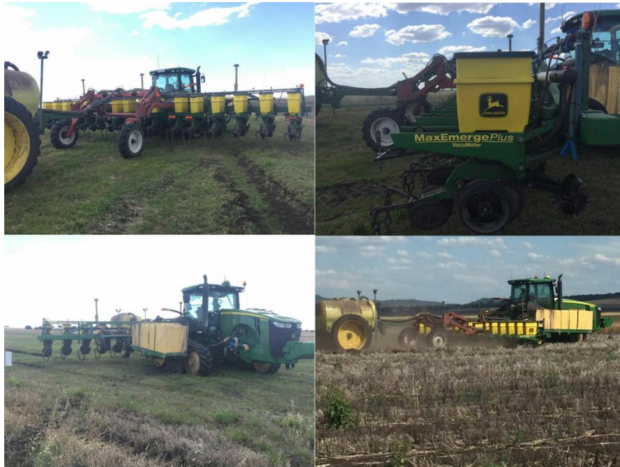
Figure 3-11: Machinery unit (JD 8310 RT with MaxEmergePlus pneumatic planter) during sorghum planting operation at Evanslea site
