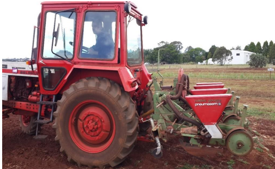
Figure 3-9: Machinery unit (Belarus 920 tractor with Nodet Gougis Pneumasem II planter) during sorghum planting operation at Ag plot site
