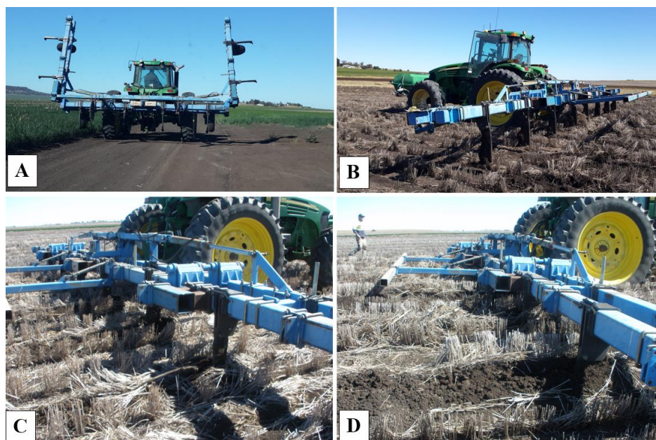
Figure 3-21: Evanslea site: (A) Folded Tilco eight tines ripper on the road, (B) On the experiment field's soil, (C) During (D1= 0 - 0.3 m), and (D2 = 0 - 0.6 m)
