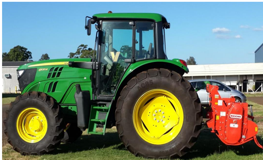
Figure 3-14: Machinery unit (JD 6105 M with Maschio FRESA B 205 rotary hoe) before softening the Ag plot soil surface
