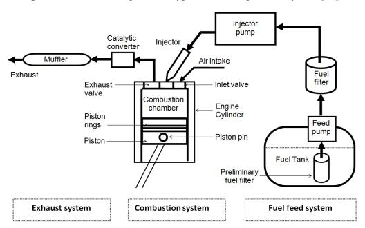
Figure 7. Schematic diagram of a typical diesel engine fuel system [12].
