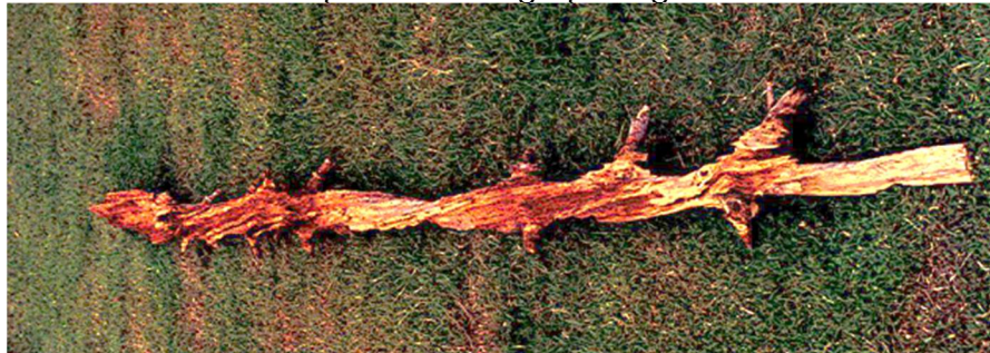
Figure 1 Spiral grain with 1.5 turns over a 4.2 meter length in slash pine.
