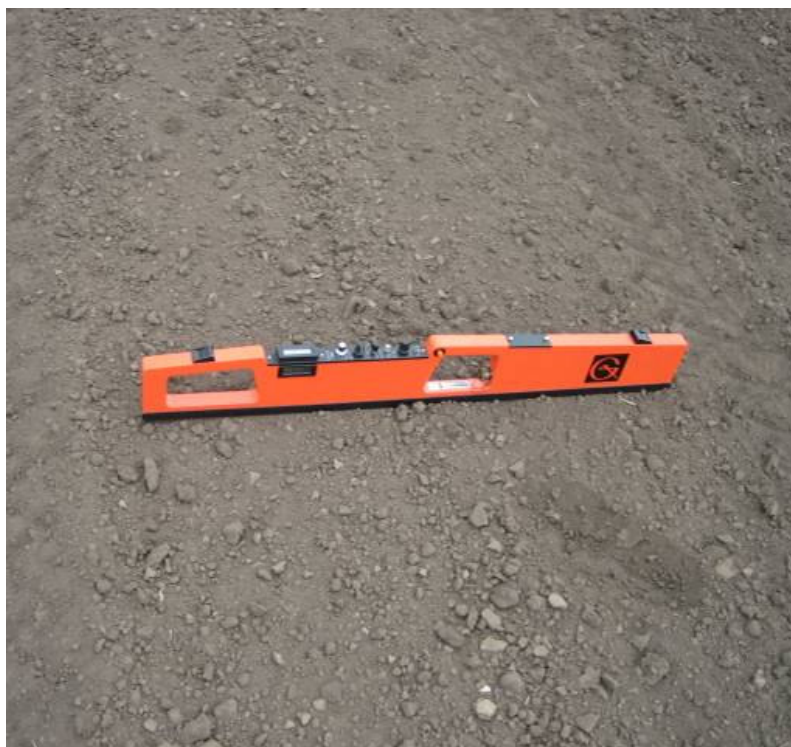
Figure 6.1 EM38 in operation placed on the soil surface (autumn trial)
