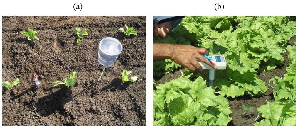
Figure 4.13 (a) Tensiometer installed next to each catch can and (b) soil tension measurement
