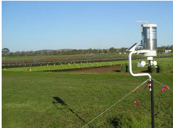
Figure 4.3 Weather station installed near the trial site
