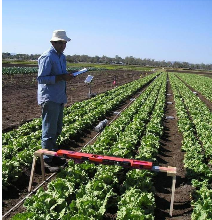
Figure 6.2 Use of EM38 on wooden stand (winter trial)
