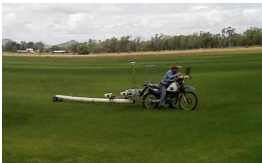
Figure 2: NDVI and EM38 mounted on an Ag-bike
