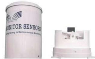
These digital rain gauges provide reliable measurement of rainfall and intensity using the tipping bucket principle. The design includes several features to maintain accuracy of measurement, including a syphoning device which "smooths" the flow of water through the system thereby minimising errors associated with varying intensity of rainfall.
