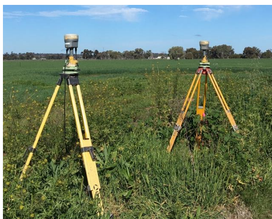
Figure 6: Field data collection using GNSS receivers
