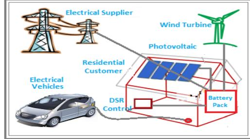
Fig. 6. Power flow of demand side response smart grid system integrating on-site renewable energy sources and electrical vehicles
