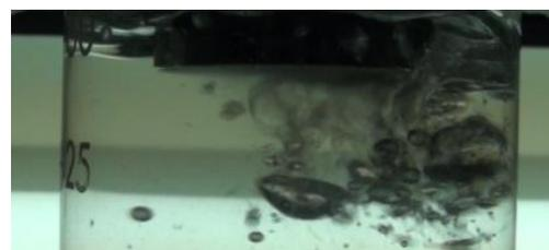
**Figure 5.** Generation of large bubbles in the suspension with ultrasonic intensity of 24.17 W/cm<sup>2</sup>.
