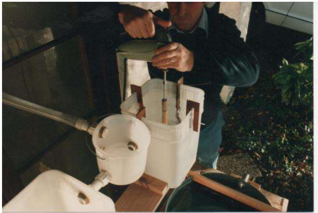
Plate 8.2: Pilot Plant Slow Mixing during a Batch Test
